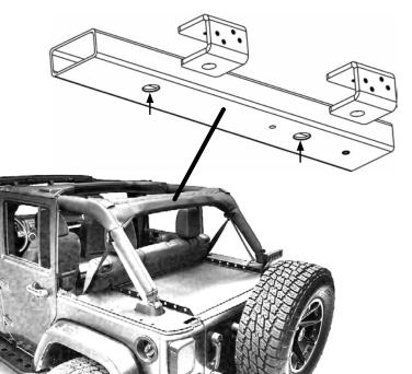
After deciding your best mounting location, slide the JL Mount over the tube keeping the counter-sunk hole facing downwards
