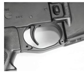
[4] While supporting the underside of the trigger guard, carefully drive in the front roll pin using the 1/8" punch. Verify the hole alignment is correct before proceeding. Roll pin should be equally flush on both sides of the weapon.
