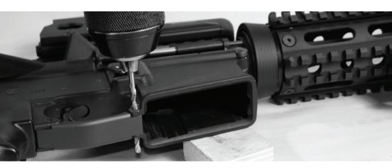
[3] Align the front hole of the trigger guard with the existing hole in the receiver. Using the No. 30 drill bit, drill through the entire trigger guard hole until the drill bit passes through the bottom side of the receiver. Make sure the trigger guard holes align. This will ensure a straight hole from top to bottom.
