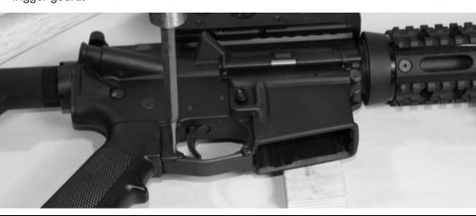
[2] Installation of the replacement guard requires you to support the underside of the trigger guard, carefully drive in the rear roll pin using the 1/8" punch. Verify the hole alignment is correct before proceeding.
