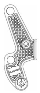
For mil-spec grips the arrow if facing up with the thinnest part of the outer shell facing up towards the trigger post.
