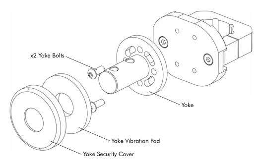
[1] Apply threadlocking fluid to the two yoke bolts and attach it to the mount base. Use whichever bolt pattern fits your application. Torque to 7 - 10 foot pounds.
