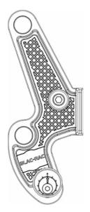
In this picture, the grip rest is set to the shortest length of pull. The arrow is facing up to the trigger post and the thickest portion of the outer shell is up towards the trigger post.
