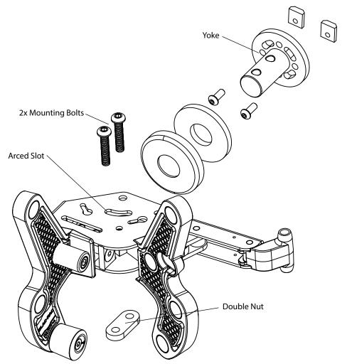
[2] Remove the yoke by pulling straight out from the unit. Remove the yoke security cover and the yoke vibration pad to access the yoke bolts. Retain for re-installation.
