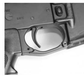
[4] While supporting the underside of the trigger guard, carefully drive in the front roll pin using the 1/8" punch. Verify the hole alignment is correct before proceeding. Roll pin should be equally flush on both sides of the weapon.
