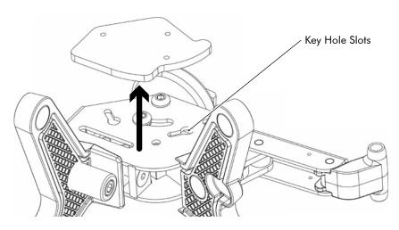
The design of the BLAC-RAC allows it be installed with up to a 45° angle from center. One of the mounting bolts is inserted through the arced slot. This slot allows for proper positioning depending on the application.
