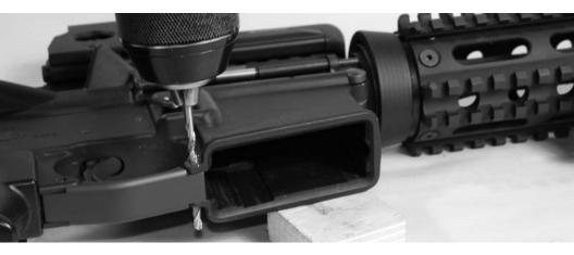
[3] Align the front hole of the trigger guard with the existing hole in the receiver. Using the No. 30 drill bit, drill through the entire trigger guard hole until the drill bit passes through the bottom side of the receiver. Make sure the trigger guard holes align. This will ensure a straight hole from top to bottom.
