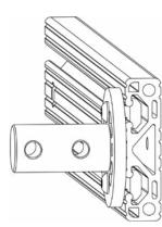
The Breech Adjustment is used to adjust the width and/or pressure of the BLAC-RAC, depending on the receiver width of the firearm being secured. The BLAC-RAC will accommodate most weapon's platforms in use by law enforcement today.
